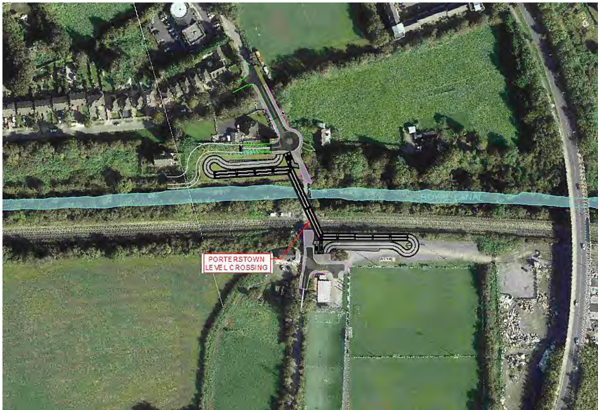
Figure 4-177 Alignment at Porterstown level crossing
