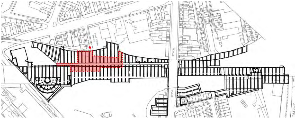
Figure 4-59 Plan view of the arches under the platforms. The area in red indicates the location to be refurbished.
