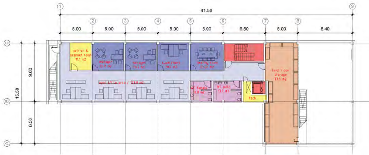
Figure 4-152 Building layout at first floor
