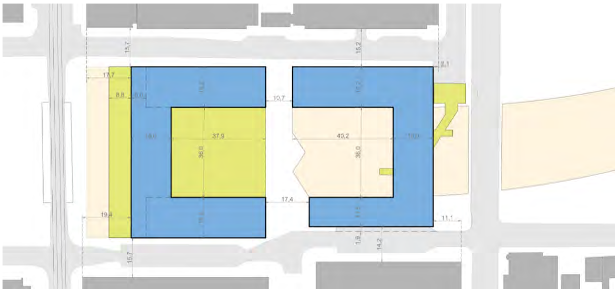
Figure 4-91 Potential arrangement of OSD (blue) integrated with the proposed Spencer Dock Station (green)
