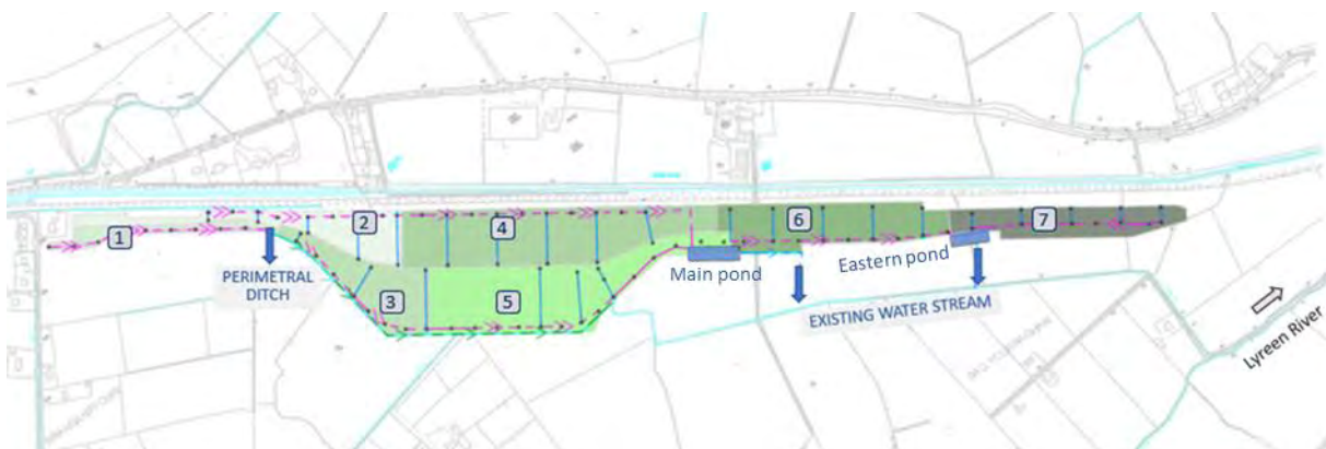
Figure 4-252 Surface drainage sub catchments
