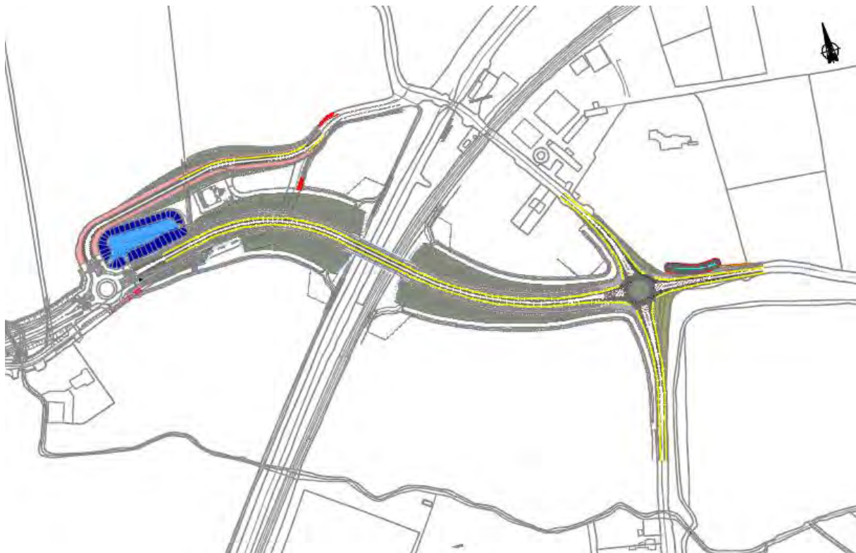
Figure 4-191 Barberstown level crossing general arrangement
